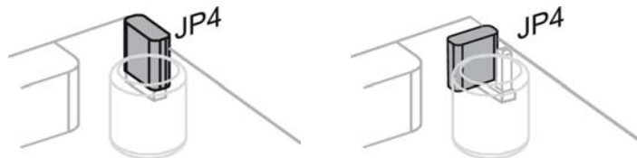
Figure 4-7 Jumper JP4 – closed (left) / open (right)
