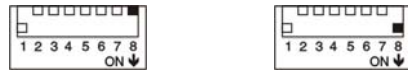
Figure 4-33 DIP Switch (JP1 [8]) – CAN Bus Termination in CAN-S (left “OFF” right “ON”)
