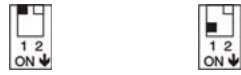
Figure 4-31 DIP Switch (JP1A) – CAN Bus Termination in CAN-M (left “OFF” right “ON”)
