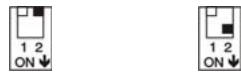
Figure 4-32 DIP Switch (JP1A) – CAN Bus Autobitrate in CAN-M (left “OFF” right “ON”)
