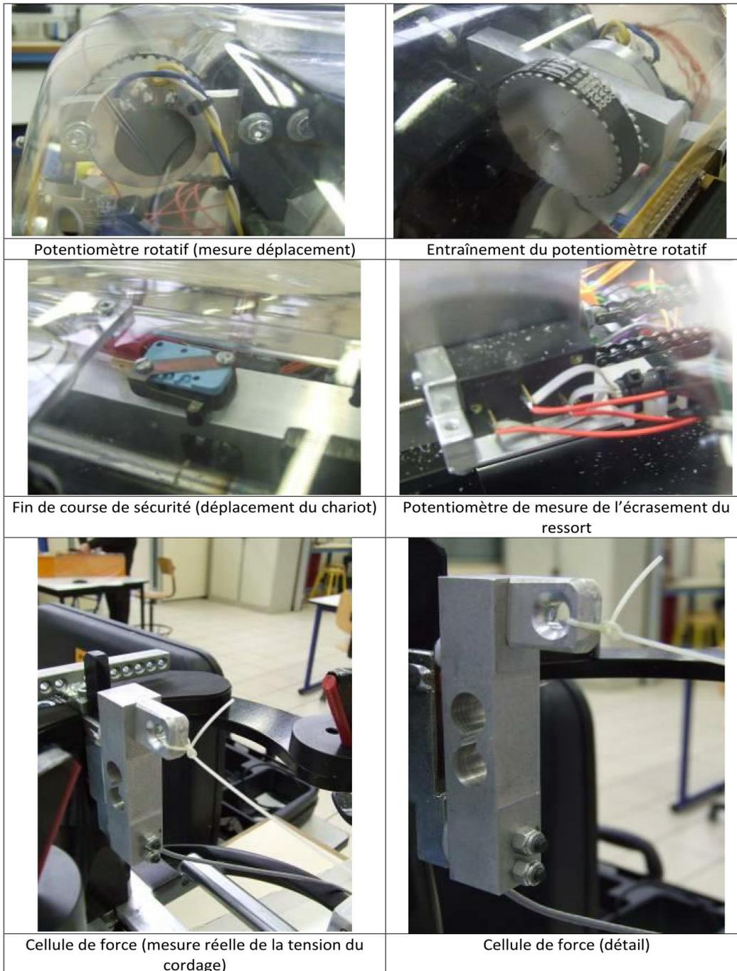
**DISPOSITIF DE MESURE DE LA TENSION DE LA CORDE DU SYSTEME DE MISE EN TENSION :**
